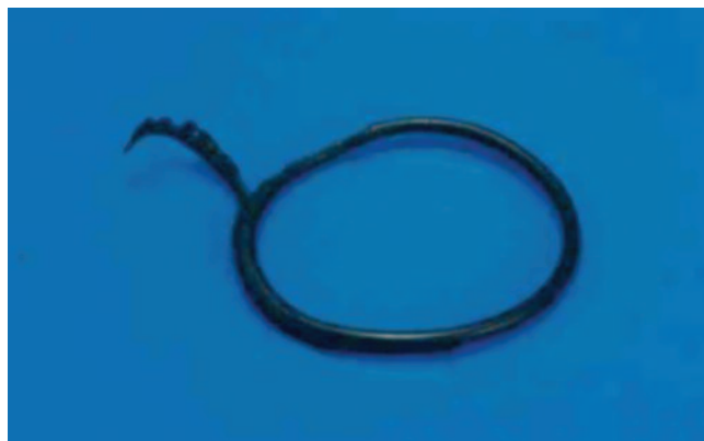
Figure 5 – Typical examples of extrusion failure
