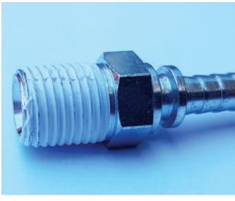
Irrespective of what sealant is used do not allow sealant to overhang the end of the male thread.
