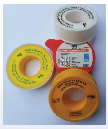
The width of tape size must be suitable for the size of the male tapered thread being sealed. It is common to use tape which is 1/4" wide when sealing 1/8", 1/4" and 3/8" taper threads and 1/2" wide when sealing 1/2" and larger diameter taper threads.
