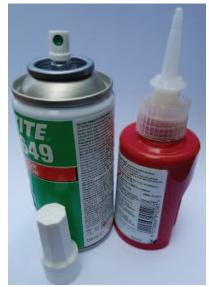
Anaerobic adhesives work by completely filling the gaps between the mating male and female thread form. Using an anaerobic sealant prevents loosening from vibration and also protects the joint from corrosion which can result from the ingress of moisture.
